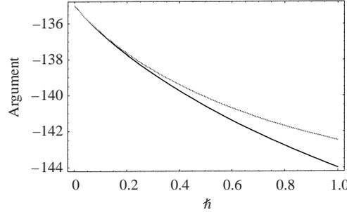
FIGURE 17. Argument of  $\bar{\phi}'_1$  for  $\hbar = 1/3$  as a function of  $Re_s$ : black line, with lift; grey line, without lift.
