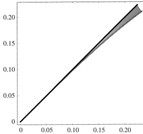
FIGURE 2.  $\tilde{\phi}_1$  branch of  $\lambda$  for 100 equally spaced values of  $\omega$  ( $= Re_s/9\hbar$ ) in the range  $[0.001, 0.1]$ . Thick black line:  $\{Re^{i\pi/4} : R > 0\}$  and thick grey line:  $(\sqrt{2}/2)\sqrt{-1 + \sqrt{1 + 4i\omega}}$ .
